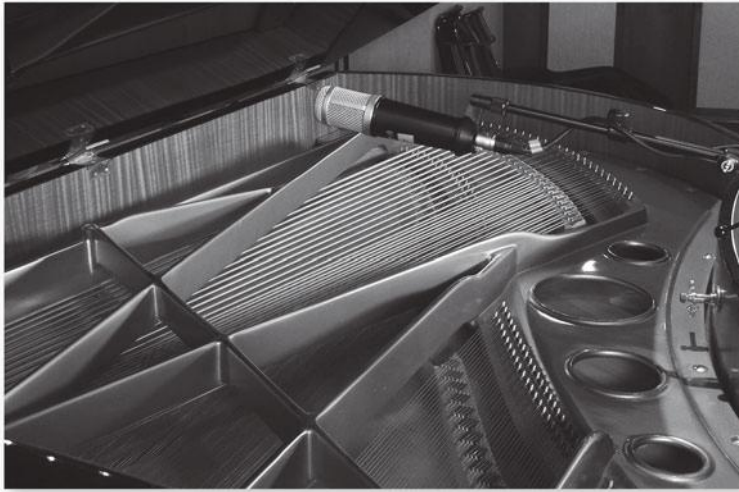
FIGURE 6.11 You can bring more of a grand piano's strings within range of a single close mic by positioning it where the mid- and low-register strings cross over.
