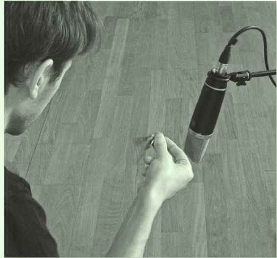
FIGURE 6.21 Recording a jangling bunch of keys is a revealing test for any microphone.
