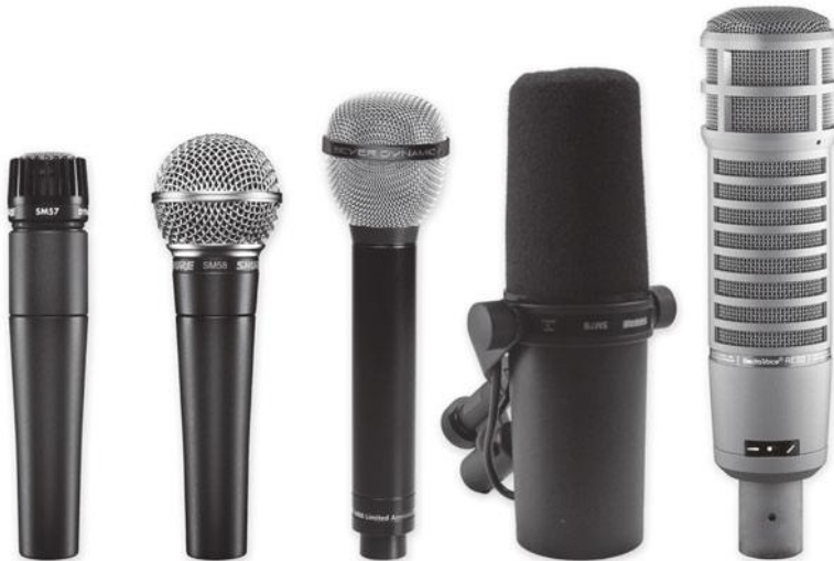
FIGURE 5.3 Some of the most enduringly popular dynamic mics for vocal recording (left to right): Shure SM57 and SM58; Beyerdynamic M88; Shure SM7; and Electrovoice RE20.
